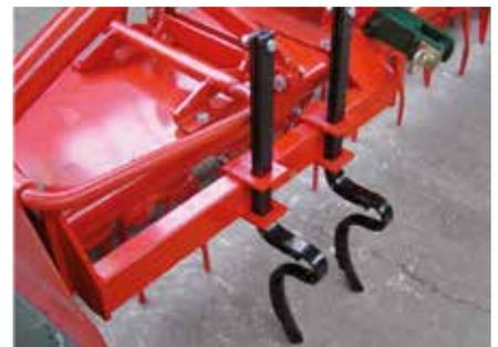
All Beyne rotary harrows are equipped with adjustable track looseners. This option loosens the tramlines behind the tractor wheels and avoids irregular soil compaction.
