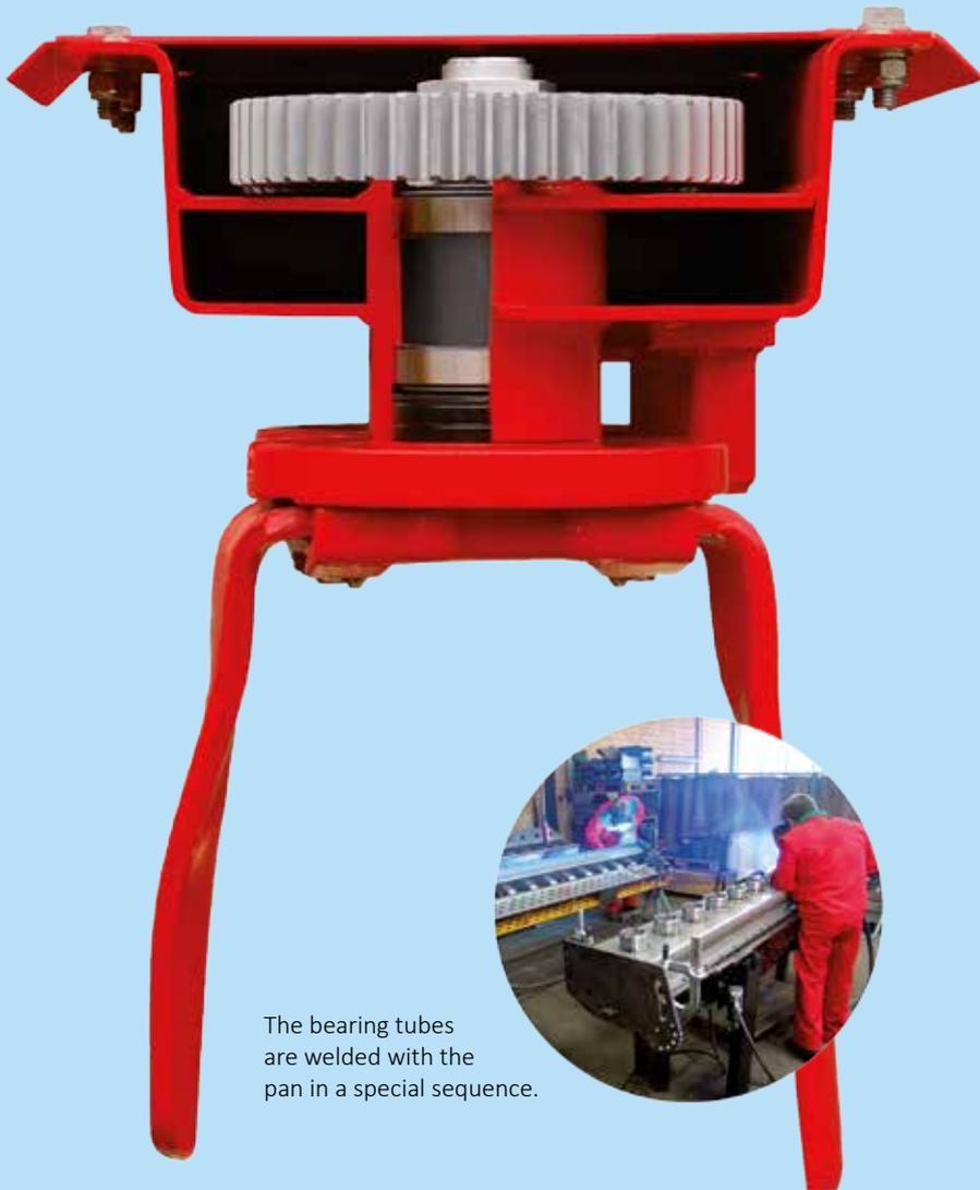
The bearing tubes are welded with the pan in a special sequence.
