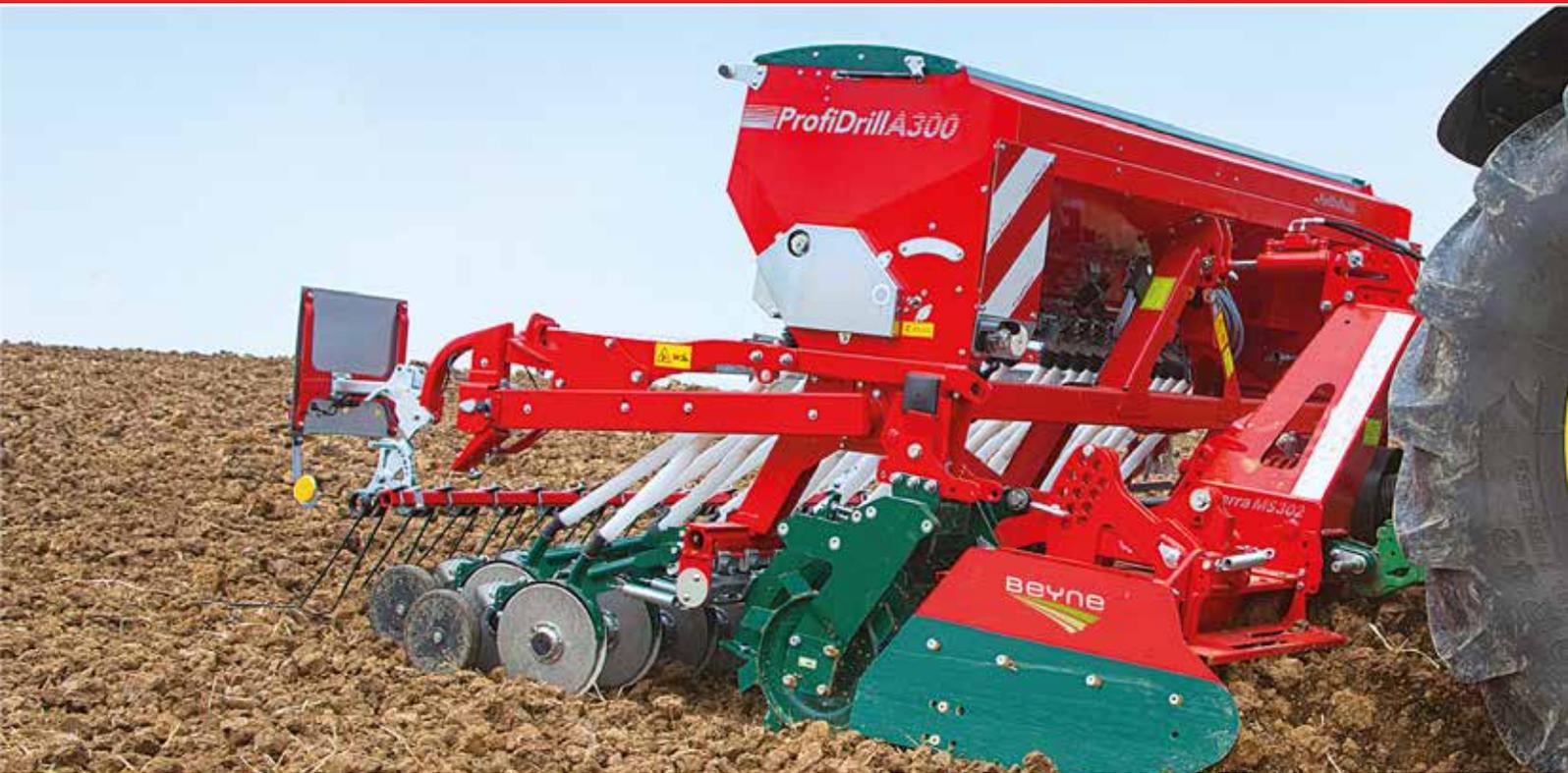
Arterra MS 302 with crumbling packer roller combined with attachment seed drill ProfiDrill A
