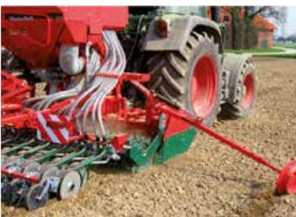
The Terramat and Arterra rotary harrows can also be fitted with track indicators for use with the seed drill. These are operated by a double-acting hydraulic system and fold vertically.
