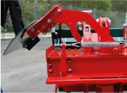
The stable side plates are double conducted, break-proof and light weight.
