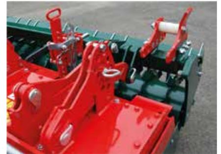
The placement of the depth adjustment at the Arterra machines takes place by a fine adjustment perforated plate with a coupling pin.
